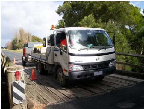
Bridge under test using small truck
