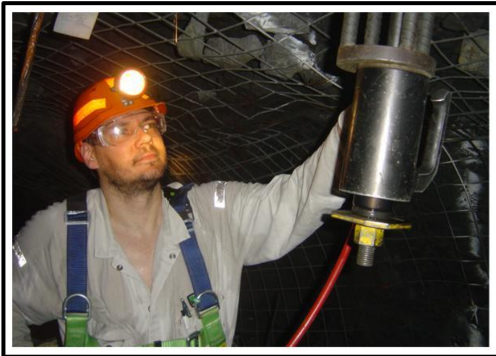
Fig 1 – Hydraulic Pull testing device used at the George Fisher Mine.
